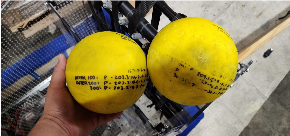
Figure 3: Higher Spring Rate ball at 375 cycles (right)
